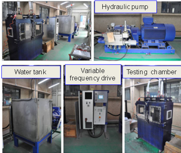
Fig.2. The equipment for offline erosion pattern test.
