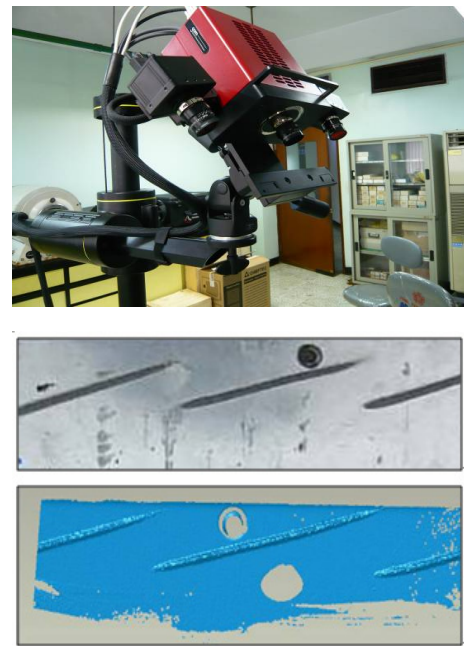
Fig.4. 3D scanner for capturing the 3D morphology of marks on the aluminum plate.
