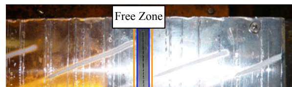
Fig.12. Free zone existing between water jet inducing incomplete descaling.
